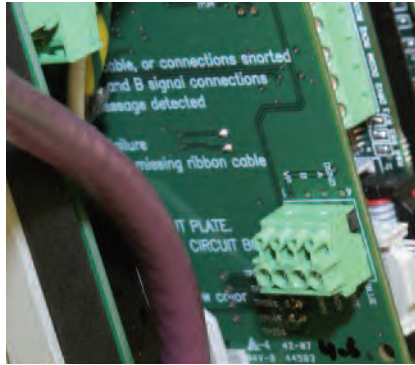
FIGURE 12-3. Profibus board showing removable 4-lead terminal block
