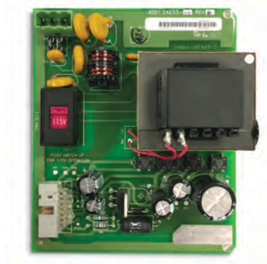
Figure 2-2: 115/230 Vac power supply (01 ordering code)
