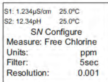
Figure 6-57: Configure Chlorine Screen
