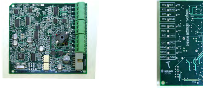
Figure 2-8: Toroidal conductivity signal board and sensor cable leads
