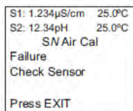
Figure 7-22: Air Cal Failure
