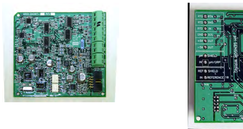
Figure 2-9: pH/ORP signal board and sensor cable leads
