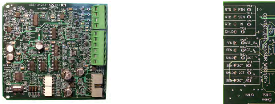
Figure 2-7: Contacting conductivity signal board and sensor cable leads
