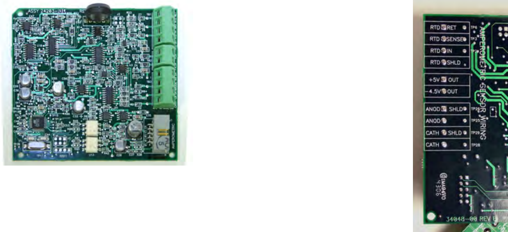
Figure 2-10: Chlorine, dissolved oxygen, and ozone signal boards and sensor cable leads
