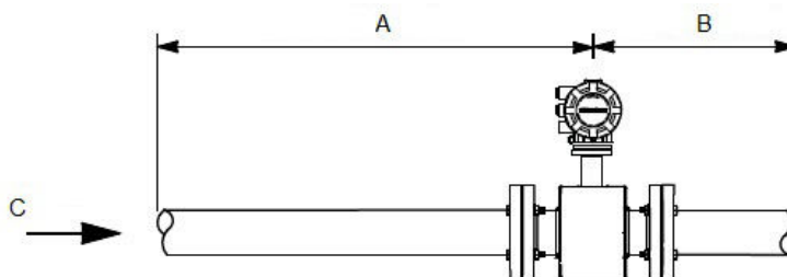
Figure 3-2: Upstream and downstream straight pipe diameters
